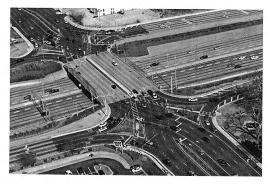
The work involves widening a half-mile of roadway plus new retaining walls, curb and gutter, sidewalks and traffic signals. The timing of other signals approaching the intersection will also get adjustments to ensure smooth traffic flow. It's estimated that the useful life of the existing bridge will be extended by about 10 years with no widening needed. The project is expected to be complete within a year.
